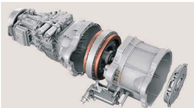
**The eTronic hybrid system is primarily designed for use in delivery vehicles requiring high levels of stop start operation.**
