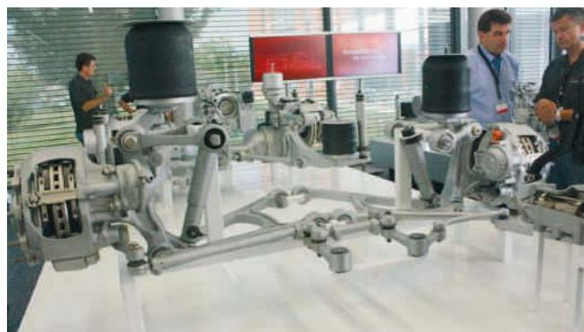
**This unit shows the standard 22.5in diameter wheel ZF IFS on the left and the new RL55 19.5in diameter wheel ZF IFS on the right.**
