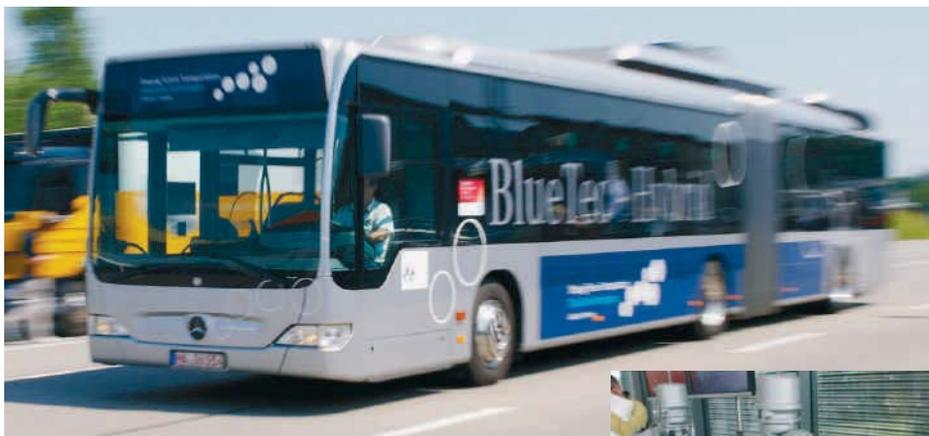
The Mercedes-Benz Citaro G Bluetec Hybrid uses the ZF AVE 130 portal axle system with hub mounted DynaStart motors. (Inset) It also uses ZF battery packs, control system and inverters. A production batch of 50 will go in to trial service in early 2011.
