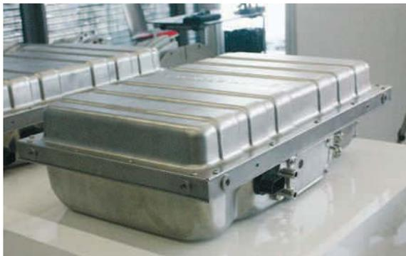
The ZF Hybrid battery pack produces 60kW. It is totally enclosed in a water cooling jacket to prolong battery life.
