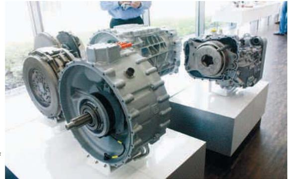
**A range of the new ZF hybrid drive units designed to be incorporated in or used in conjunction with their existing transmissions.**
