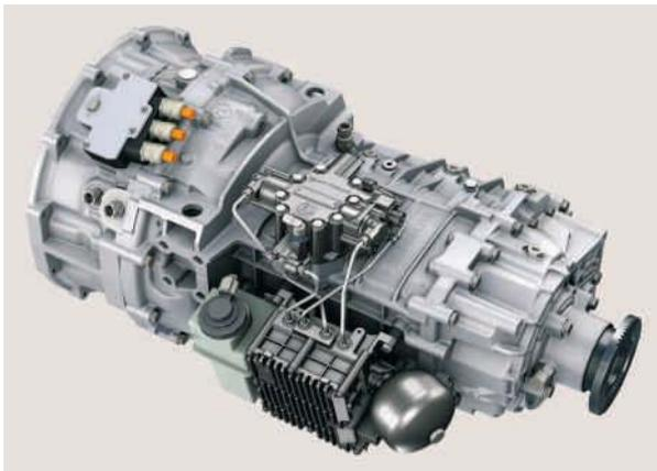
**The ZF Hytronic is a hybrid drive for vehicles up to 7.5tonnes GVW. It utilises the existing ZF AS-Tronic Lite transmission with a hybrid drive added. The AS-Tronic Lite is the automated transmission used in the Iveco Daily amongst other vehicles.**
