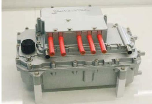
The control unit is common to all the different types of ZF hybrid.
